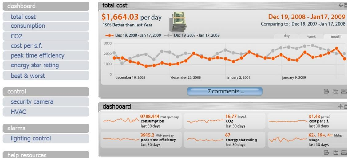
*The Luminix SmarterEnergy Web-based management interface.*
